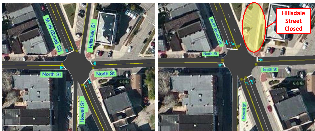
Alternative 1 – Signalize Intersection.
